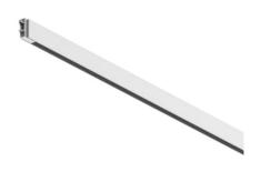
Electro-mechanical profile for indoor application with integrated direct linear light element for surface or suspended installation. With lengths varying from 1 to 2.5m (distance between ball joint centers). Fixation by a joint with power kit. Power kit and mechanical joint must be ordered separately. System controlled by 1-10V driver, DALI or Casambi. Broadcast control system. Dimmer not included.
