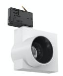
LED - LED array - 20W - 1391lm - 3500K - CRI> 97 - Beam<sup>o</sup> 15
